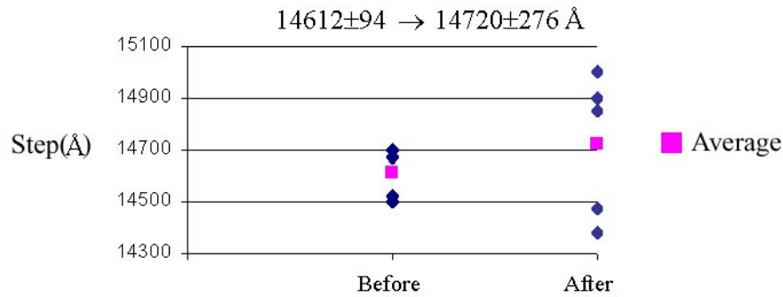
Figure 3-18. Swelling test of PPy in Au etchant for 5 min.
