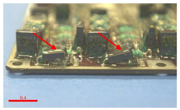
Figure 3-7: This photo shows bent components on board #2. This is done to facilitate small vertical clearances in these areas.
