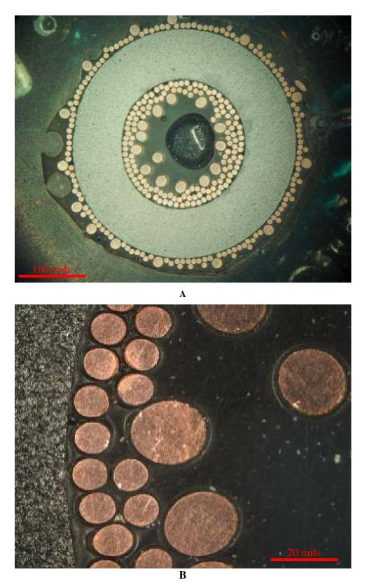
Figure 3-15: These photos show the cross-section top view of one of the transformers. B, an enlargement of an area in A, shows the separation between the coils.
