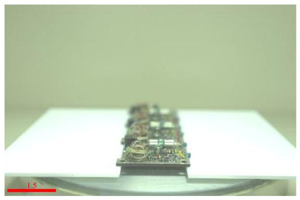
Figure 3-4: This photo shows the setup to measure board flatness. The board is suspended by its edges on ceramic plates on a flat glass plate.
