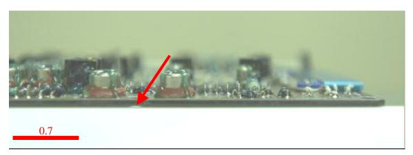
Figure 3-5: This photo shows the area where the measurement was taken for the board flatness assessment.
