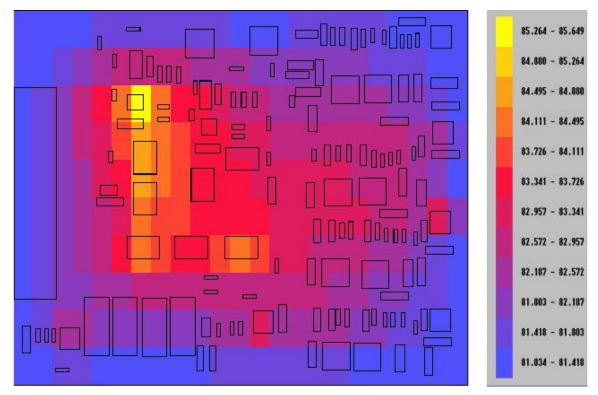
Figure 6-5: Temperature distribution across Electronics Interface (SPA) at 81° C.
