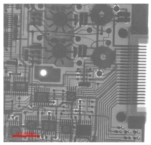
Figure 3-11: This X-ray image shows the layout for board number 2559023 in the area containing the two transformers that were removed for the DPA.
