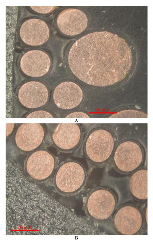
Figure 3-16: These photos show the cross-section top view of one of the transformers. In B, it can be observed that there are voids between the coil wires.
