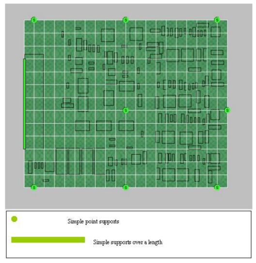
Figure 6-6: Position of supports for Electronics Interface
