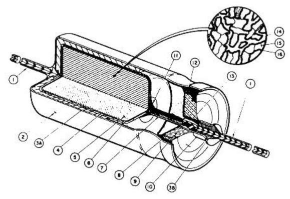
Figure 3-12: This schematic shows a typical solid tantalum capacitor (MIL-STD-1580A).
