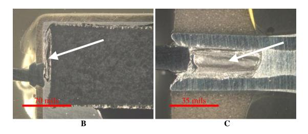
Figure 3-14: These photos show the cross-sectional side overview of one of the tantalum capacitors (A). In B a void in the solder in the around the tantalum plug can be seen. In C a void in the solder in the tubulet is shown.
