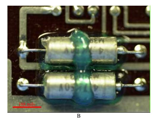
Figure 3-8These photos show the location on board number 2559017 from where the two capacitors for the DPA were removed (see red box in A). Figure B shows an enlargement section with the two capacitors.
