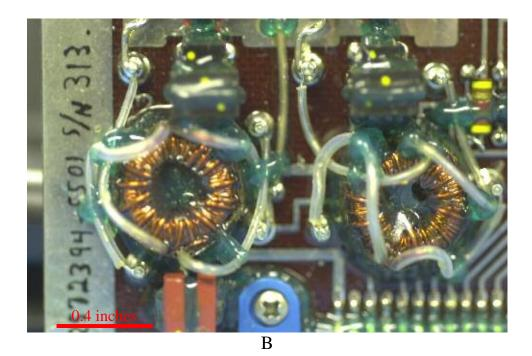
Figure 3-9: These photos show the location on board number 2559023 from where the two transformers for the DPA were removed (see red box in A). Figure B shows an enlarged section with the two transformers.
