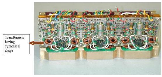
Figure 6-3: Power Switch Driver Off board
