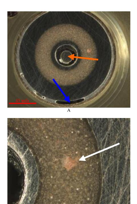
Figure 3-13: These photos show the cross-section top view of one of the tantalum capacitors. In A, it can be observed that the pin is not exactly centered, and that there are some voids in the solder. B is an enlargement of an area in A where a reddish discoloration was seen in the glass seal.
