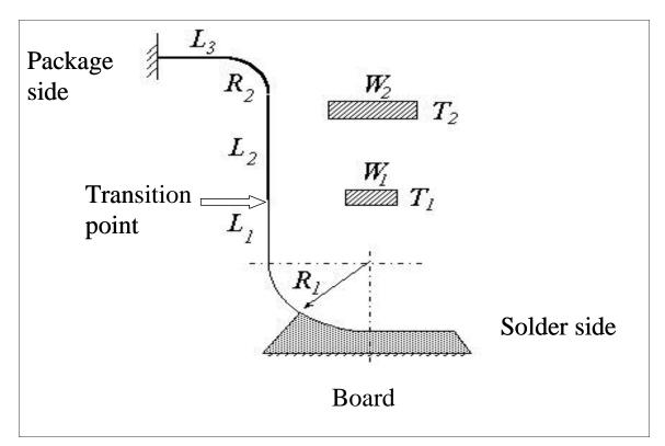
Figure 6-2:Interconnect dimensions for gullwing components
