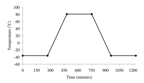
Figure 4-2 Qualification temperature cycle
