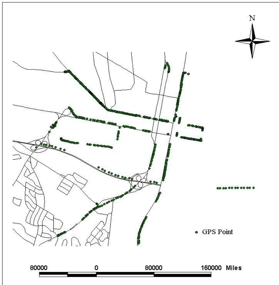
Figure 50 – Map of Part of Northern Virginia Showing Probe vehicle tracks as recorded by GPS
