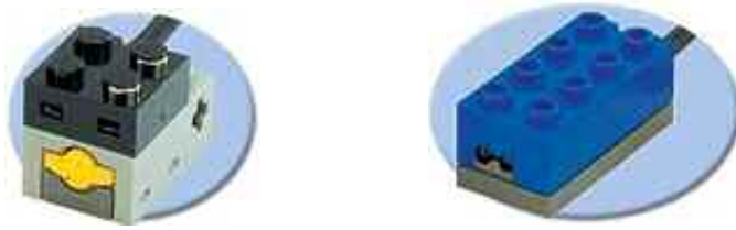
Figure 71. LEGO touch sensor (left) and light sensor (right); (taken from [118])
