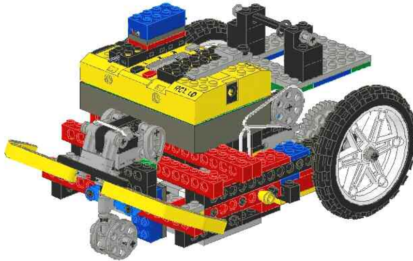
Figure 81. Pen holder, bumper, and RCX subsystems added to assembly
