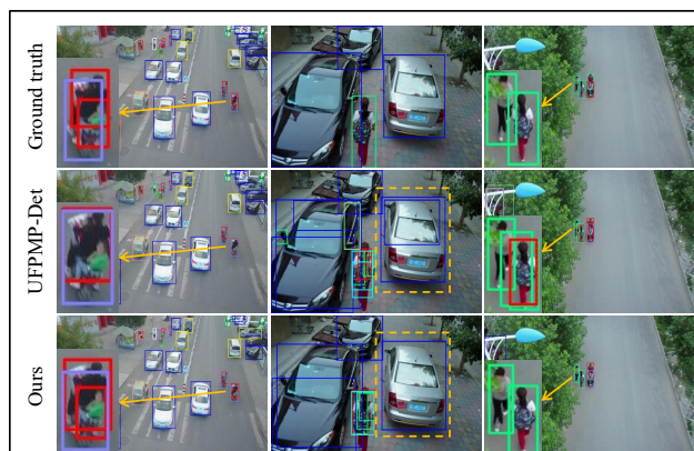
Fig. 8 Qualitative results on VisDrone (Person, Motor, Car, Pedestrian). Incorporating cross-fusion successfully retrieves missed small objects (indicated by arrows) and eliminates false alarms (indicated by dotted boxes) by the UFPMP-Det baseline.
