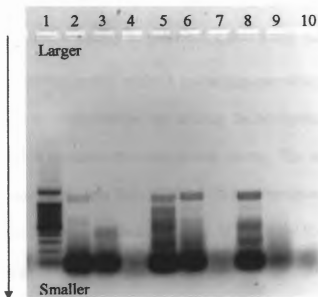
Figure 13. Sample agarose after electrophoresis has been run. Lane 1 contains the standard and lanes 2-10 have different conditions with a primer pair.
