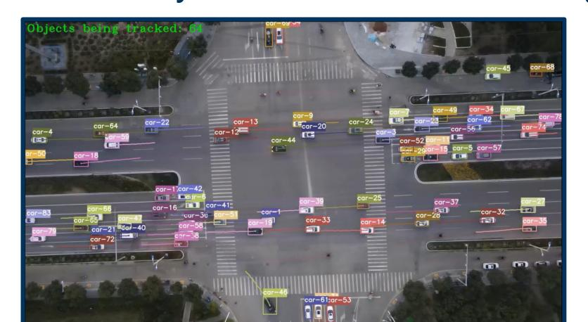
The UAV data is used to model and evaluate roads and intersections, as well as predict flow under ideal conditions in order to establish a multi-scale simulation evaluation and prediction mechanism and achieve complementary calibration of realistic and ideal situation data.
