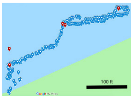
Figure 6. Path MARCo took during 5-waypoint testing at Eagle Lake. A waypoint is a specific location on Earth given in latitude and longitude. A longer path can be broken down into multiple waypoints. Between waypoints, the algorithm finds the shortest path between two points (current location and next waypoint) and tries to stay on that path. Waypoints play a crucial role in breaking the total path into smaller, shorter paths for the algorithm.
