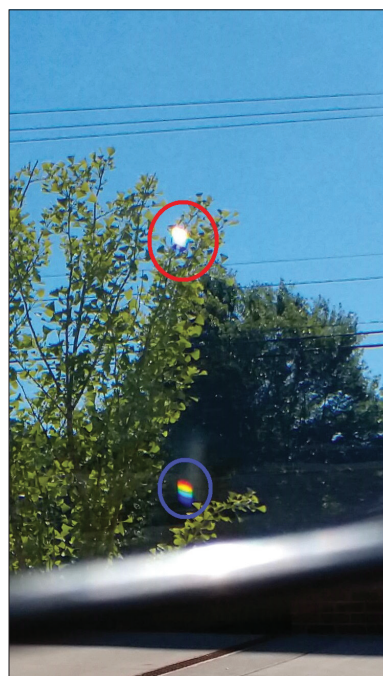
Fig. 7. An image showing the first (top red circle) and second (bottom blue circle) reflections from the back of the mirror.
