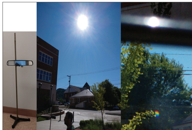
Fig. 6. A simple setup for outside observations of the Sun (right) using a ring stand with a one-meter length rod, a clamp holder, and a rearview mirror. An observer (center) locating the solar spectrum in the mirror. The spectrum observed near the bottom of the mirror after the third reflection from the back of the silvered mirror surface (right).
