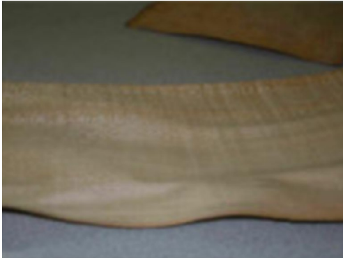
Uncontrolled and undesirable material behavior: wood veneer warps and buckles when exposed to moisture. Photo by Redbridge Marquetry Group.
