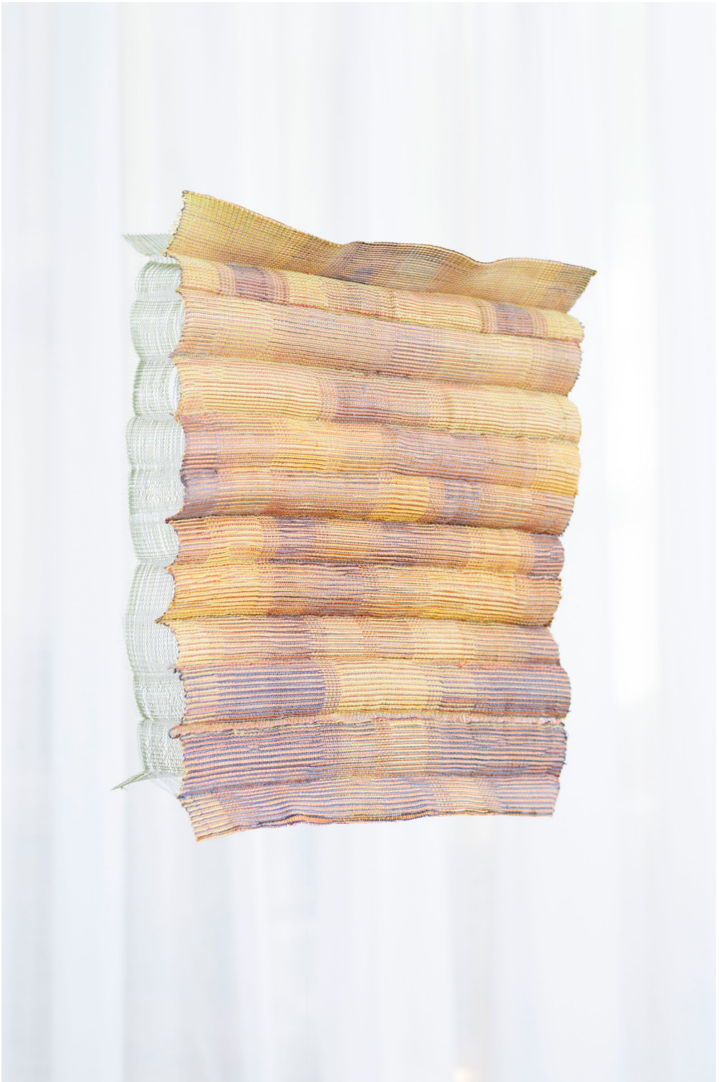
Woven spacer prototype 2 , cotton, polyester, wool and nylon monofilament yarns woven on 16-harness floor loom, 12" x 14" x 1.5", 2022.
