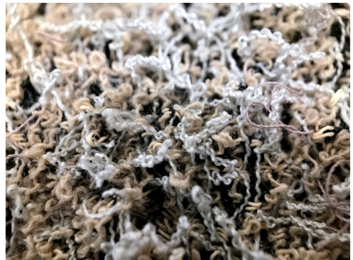
Detail of a weave structure before and after shrinking. The beige and blue elastic yarns twist back on themselves, forming a dense low-profile pile. Woven at 32 epi, 32 ppi with 1" long weft floats.
