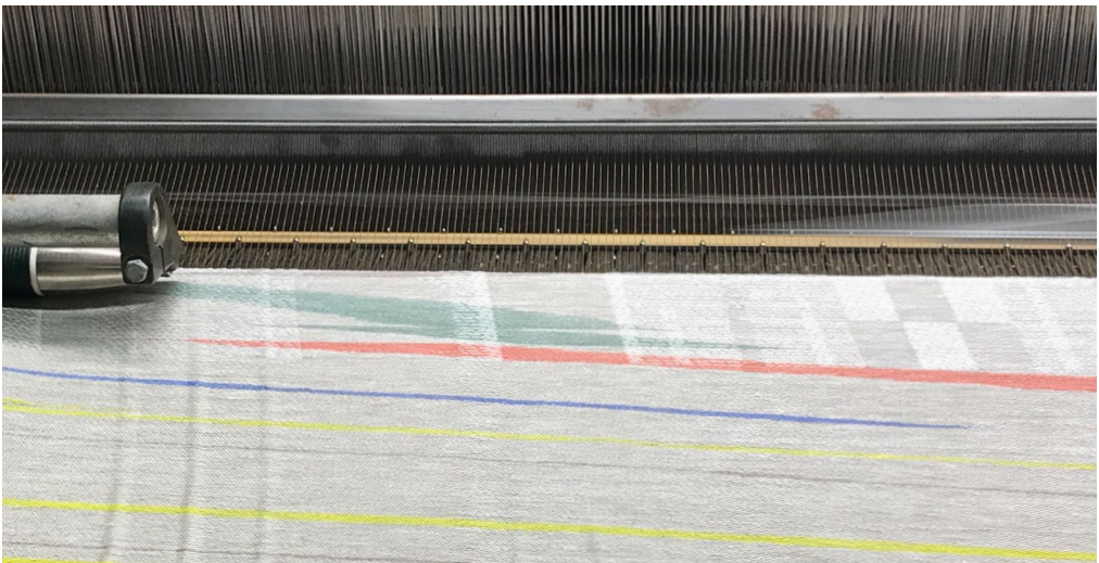
An alternative method: dyeing skeins at precise locations. This technique created irregular patches of color when woven on the Jacquard loom.
