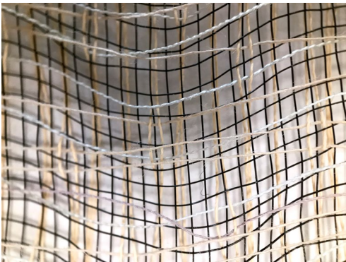
Detail of a weave structure before and after shrinking. The beige and blue elastic yarns twist back on themselves, forming a dense low-profile pile. Woven at 32 epi, 32 ppi with 1" long weft floats.
