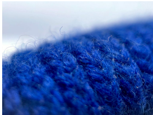
Air is present within and around loosely spun yarns, acting as a thermal insulator.
