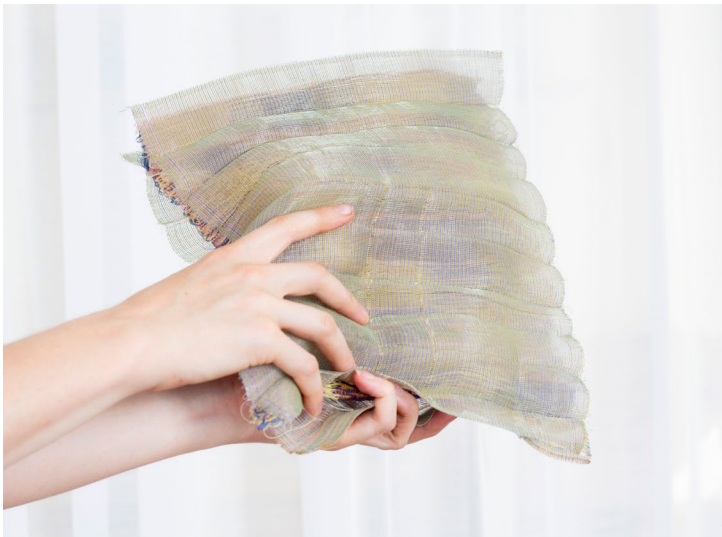
Testing the compressibility of woven spacer fabrics.
