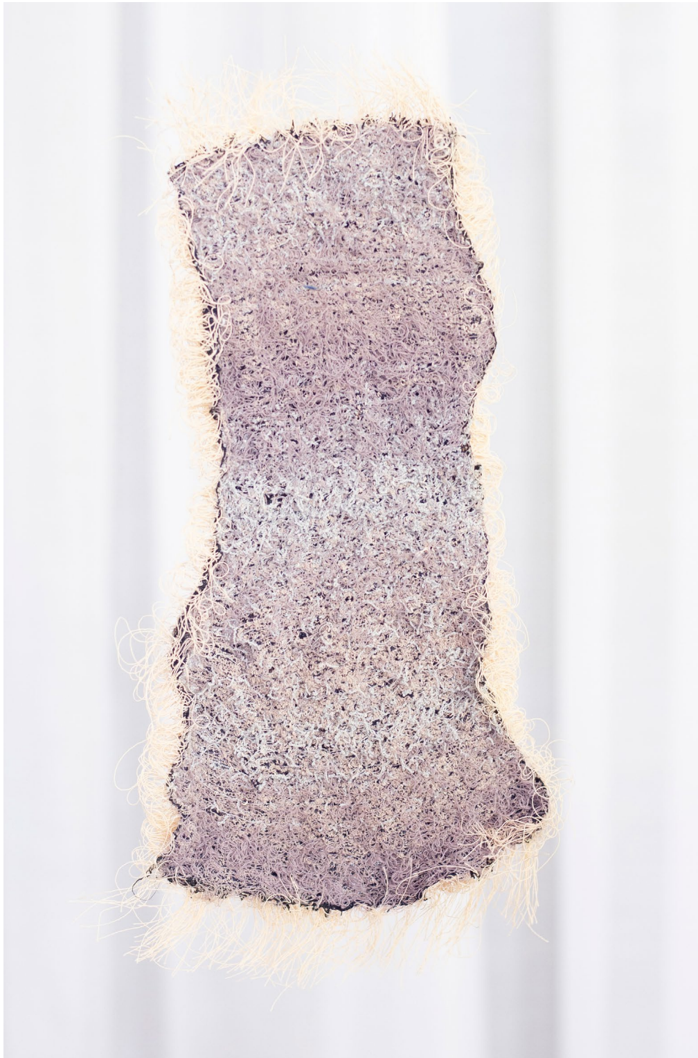
Loop-pile prototype 3, cotton, elastic cotton, elastic hemp, viscose and polycaprolactone yarns woven on 10-harness floor loom, 4" x 11", 2022.
