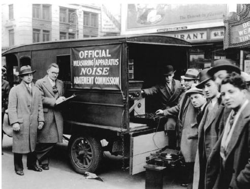
A noise-measuring van in New York City, 1930... (Property of AT&T Archives; reproduced from The Soundscape of Modernity , Emily Thompson (2002): 161.)
