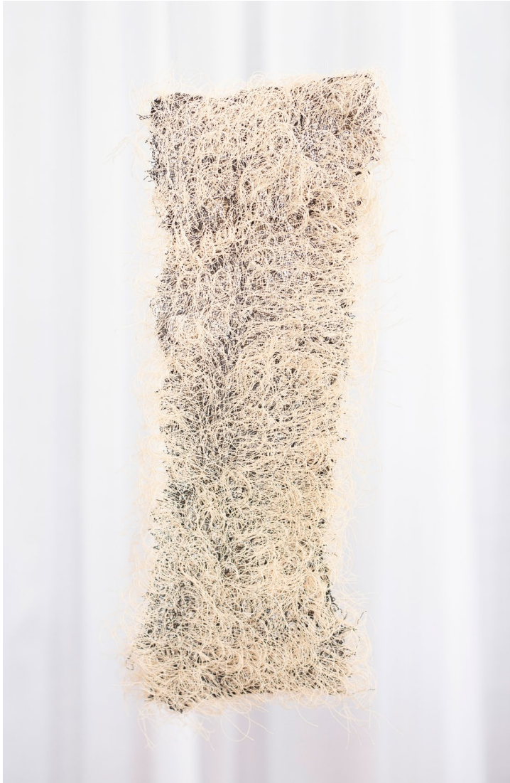
Loop-pile prototype 1 , viscose and polycaprolactone yarns woven on 10-harness floor loom, 4" x 13", 2022.
