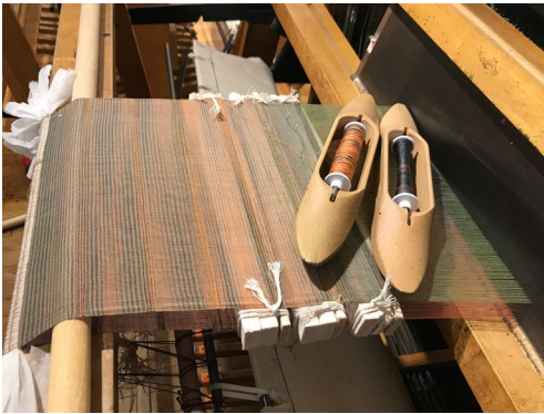
Woven spacer prototype on a 16-harness floor loom.
