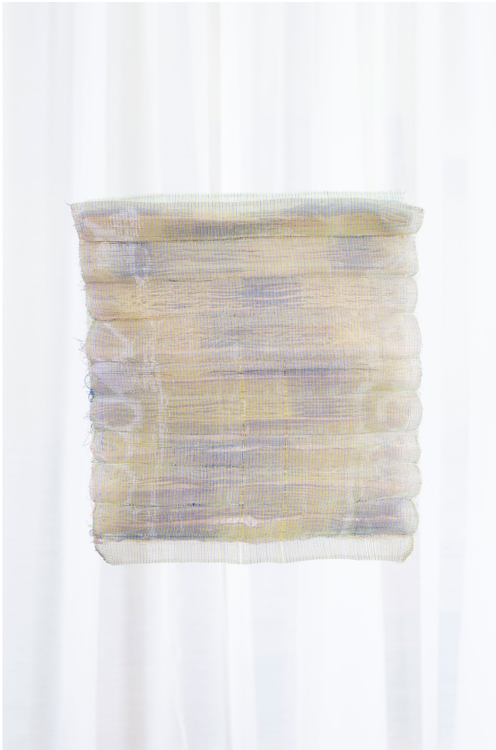
Woven spacer prototype 3 , cotton, polyester, wool and nylon monofilament yarns woven on 16-harness floor loom, 12" x 14" x 2.5", 2022.
