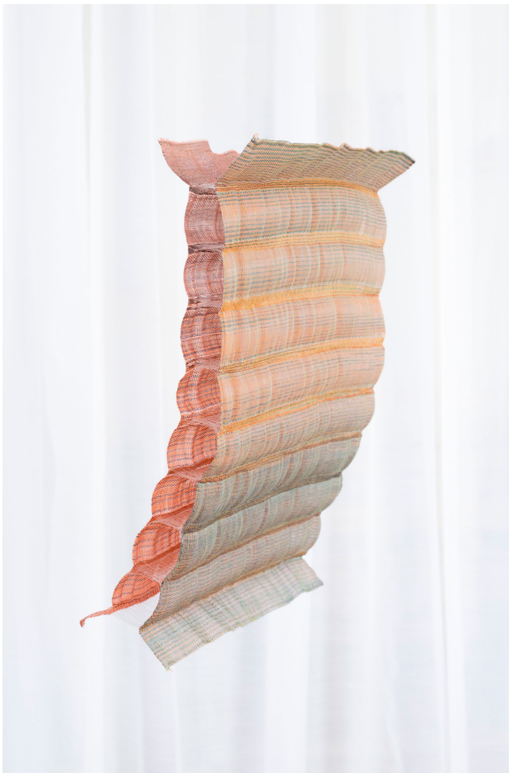
Woven spacer prototype 1 , cotton, polyester and nylon monofilament yarns woven on 16-harness floor loom, 12" x 16" x 1.5", 2022.
