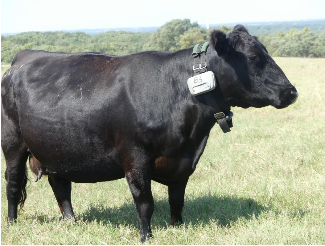
Figure 2.3: Virtual fencing collar version 2, on animal.
