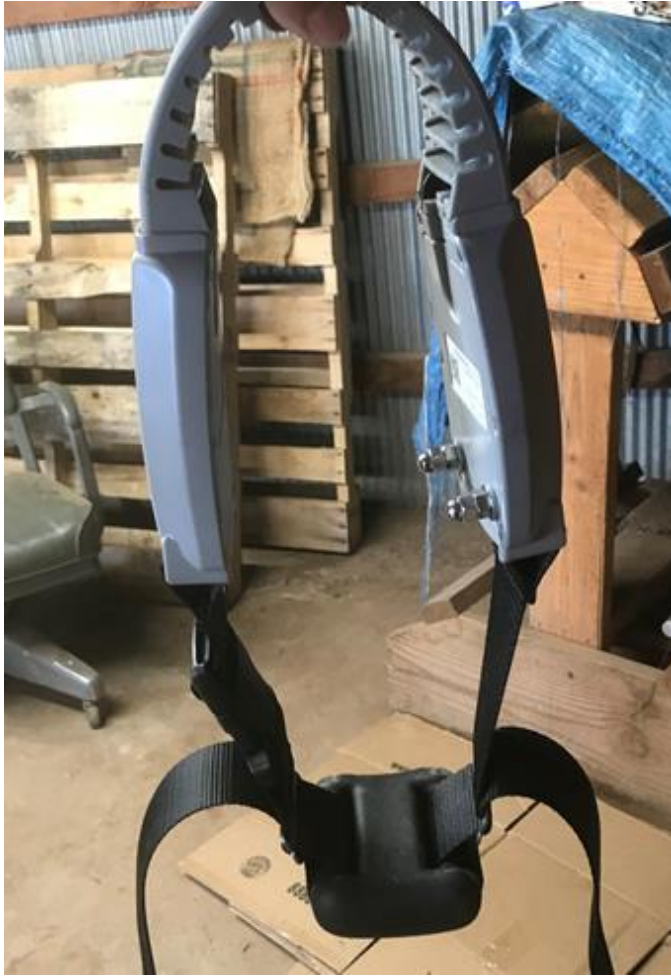
Figure 2.1: Virtual fencing collar version 1.
