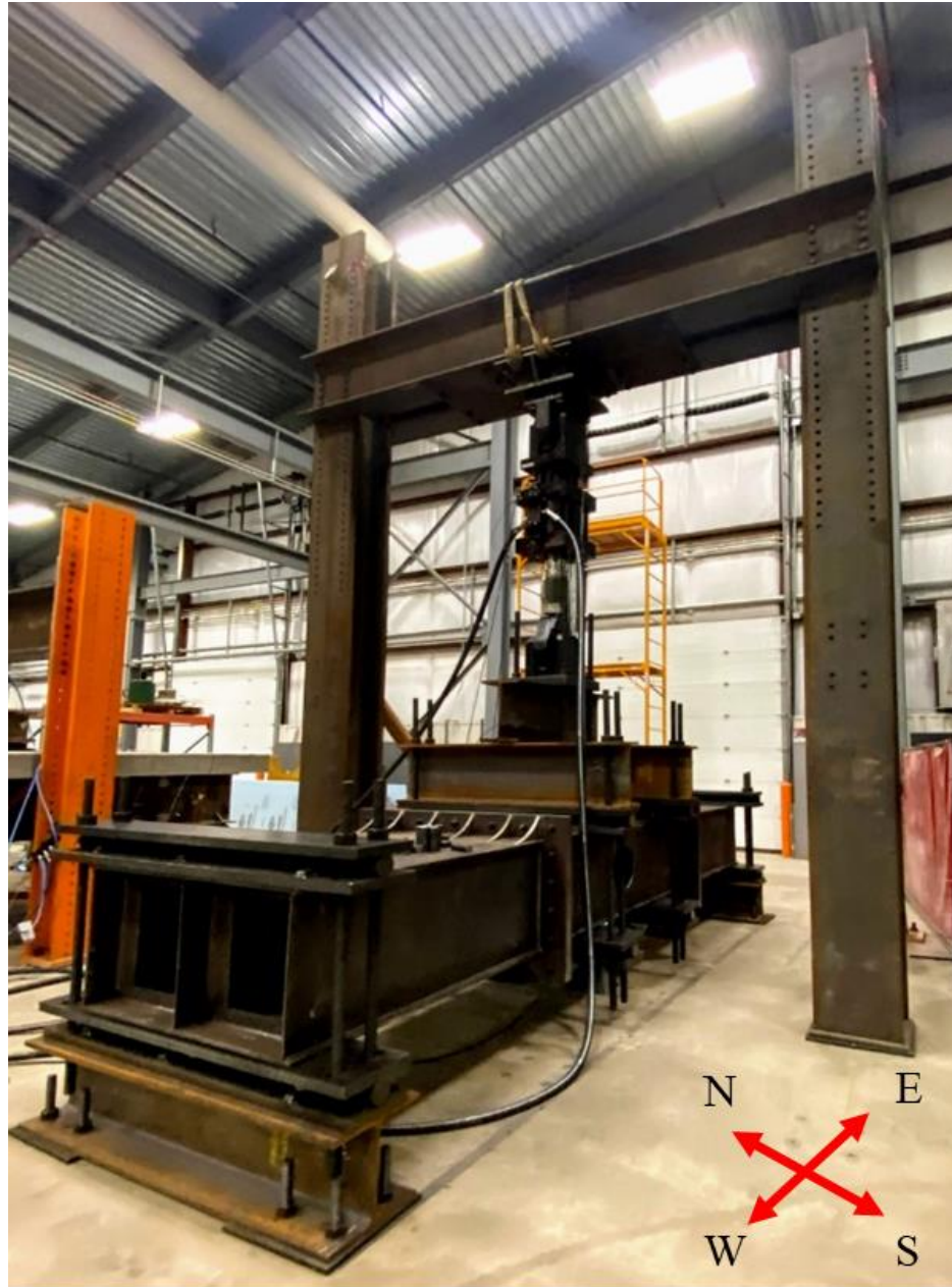
Figure 5-11. Constructed loading frame along with assembled Specimen S1.
