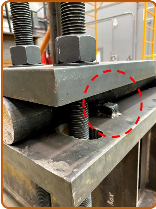
Figure 5-10. Details of hinge and roller supports in Specimen S1.
