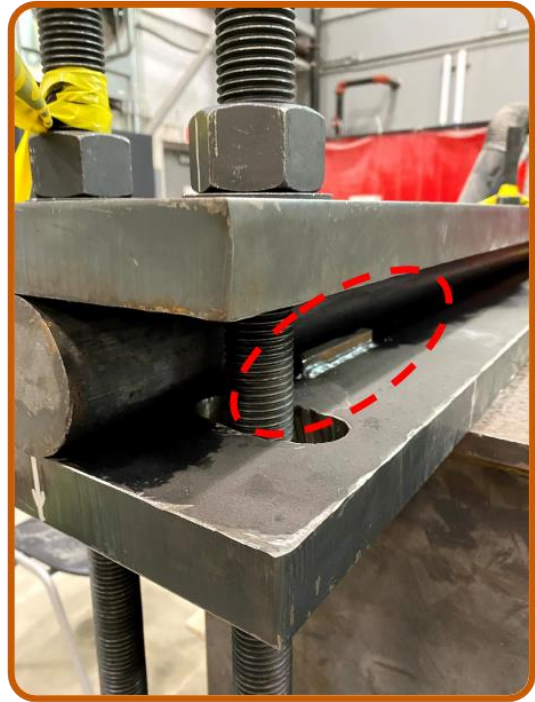
Figure 5-10. Details of hinge and roller supports in Specimen S1.
