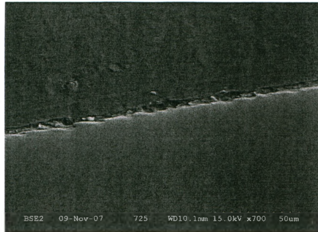
Figure 5.6 SEM close up of the surface finishes for both the flat surface (top side) and extruded profile (bottom side).
