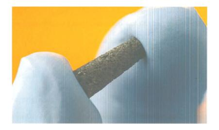
Figure 1-1: Prototype of Porous titanium foam dental implants
