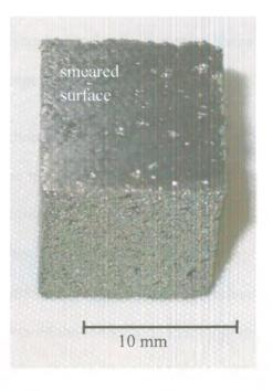
Figure 2-4: Quasi-total porosity closure in porous titanium as a post-machining effect.
