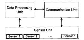
Figure 4.1: The Structure of Wireless Sensor Boards
