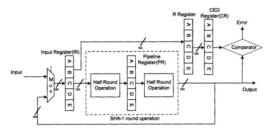
Figure 3.5: Time Redundancy for SHA-1 Hash Functions
