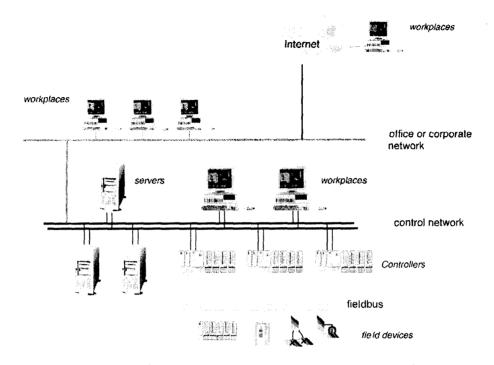
Figure 2.2: CIM(Architecture of Modern Control Networks)
