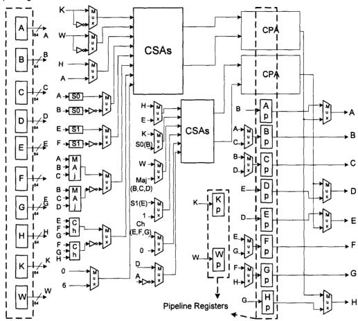
Figure 3.10: Pipelined SHA-512 Round and Inverse-Round Computation
