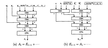
Figure 3.6: Carry-Save-Adder tree for SHA-1 round operation (operands are 32 bits long)
