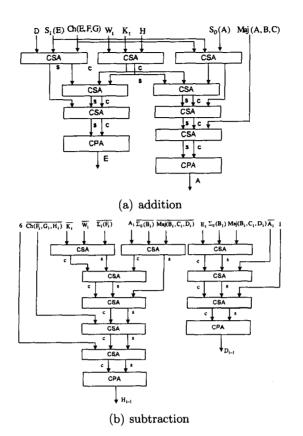
Figure 3.9: Carry-Save-Adder tree for SHA-512 round computation
