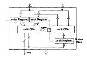
Figure 3.7: 32-bit Pipelined Carry Propagate Adder
