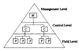
Figure 2.1: CIM(Computer Integrated Manufacturing Architecture)
