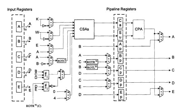
Figure 3.8: Pipelined SHA-1 Round and Inverse-Round Computation
