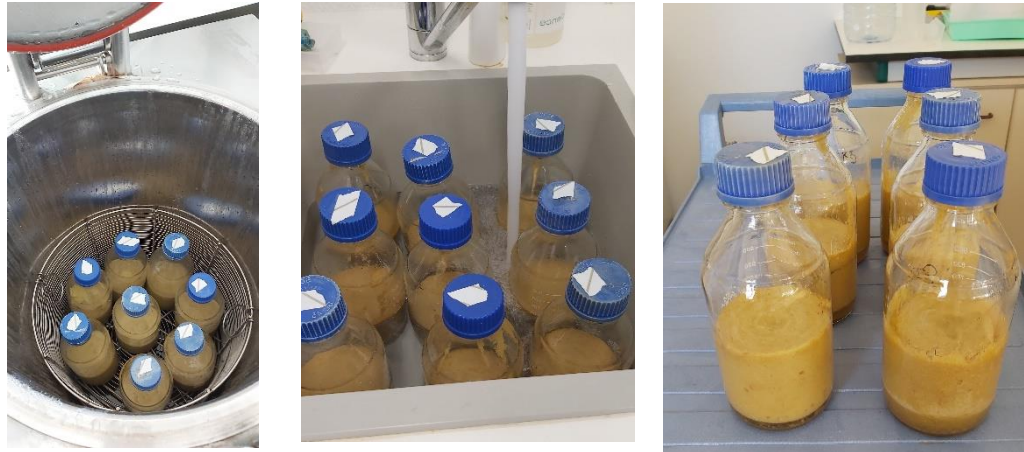
Figure 3.4 - Heat treatment of the pulps (autoclave) before starter inoculation. From left to right, samples at the autoclave and during cooling in water.
