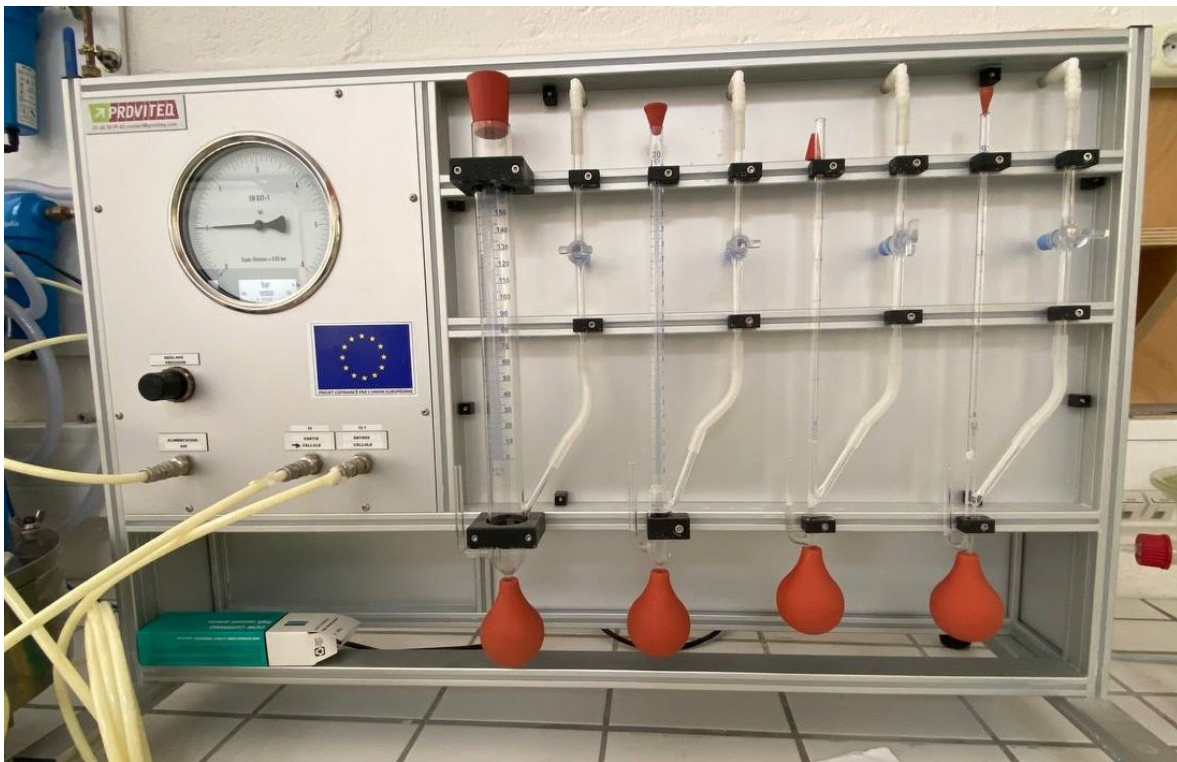
Fig. 3.9. Scheme of the Cembureau permeameter.
