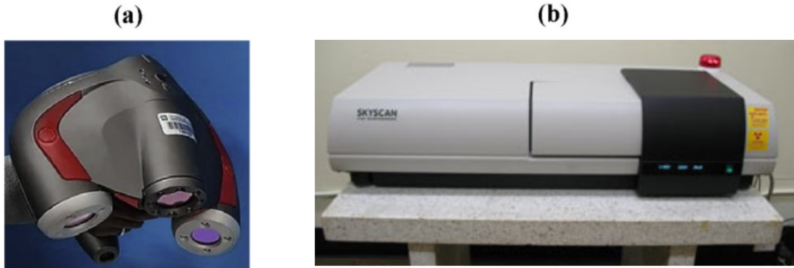
Fig. 5.2. (a) MAXscan 3D laser scanner and (b) X-ray micro-CT scanner.
