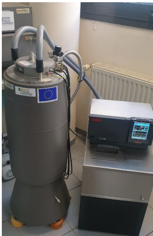
Fig. 3.10. Scheme of the Calvet calorimeter.
