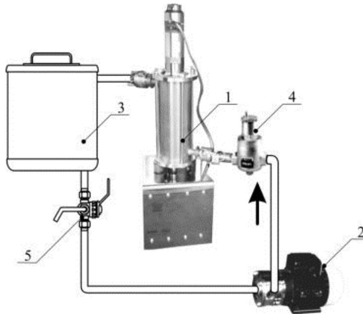
Experimental installation with the cavitational reactor of the company *Oil Tech Production OY*:
