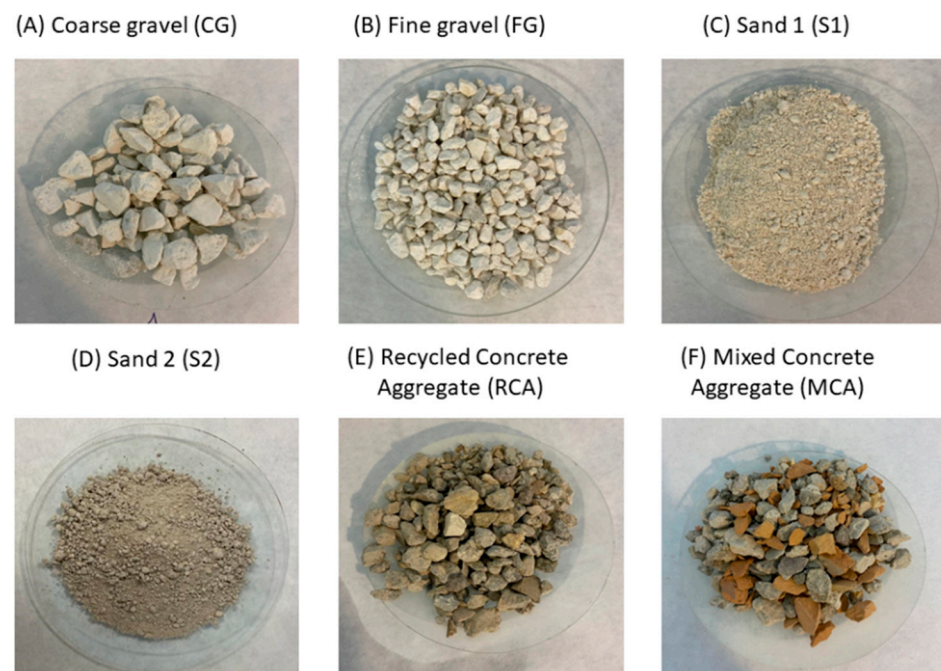
Figure 1. Images of the aggregates used (A) CG, (B) FG, (C) S1, (D) S2, (E) RCA and (F) MCA.
