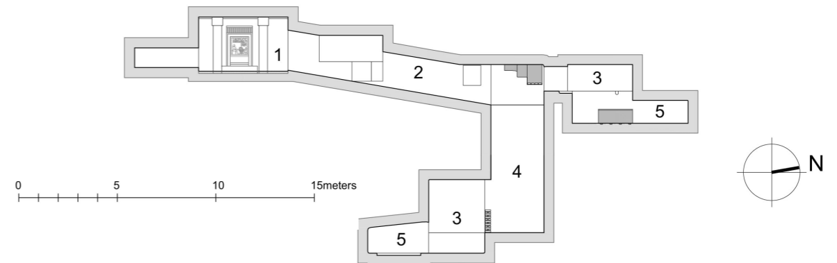
Figure 8b. Substructure of QH31. Sections: (1) cult chamber, (2) descending corridor, (3) burial chambers, (4) burial shaft and (5) burial niches. Author: J.A. Martínez Hermoso.
