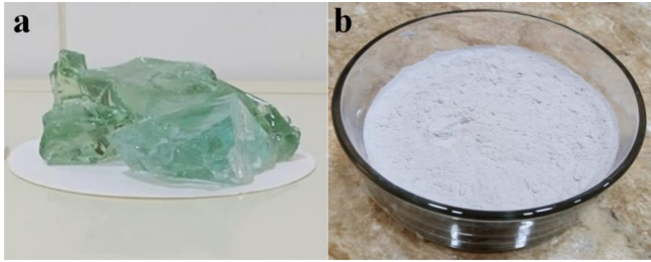
Fig. 2. a) Glass waste sample;b) Powder of glass waste to a silt size
