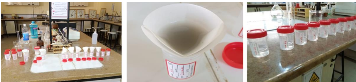
Fig. 4. The filtration of the cadmium solution from the crushed glass waste after completing the adsorption process
