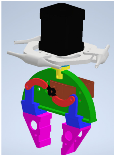
Figure 5. Moving platform with gripper
