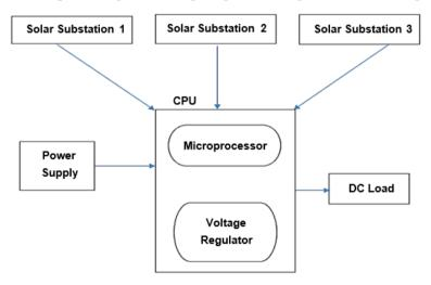
Figure 2 The block diagram of the DER system
