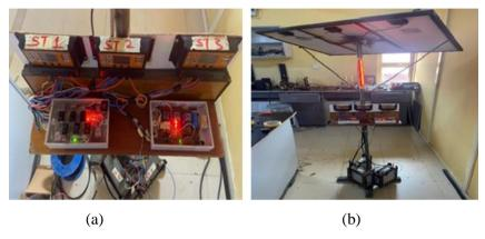
**Figure 5** The hardware units: (a) Solar Charge Controller; and (b) Assembled unit with Solar Panels
