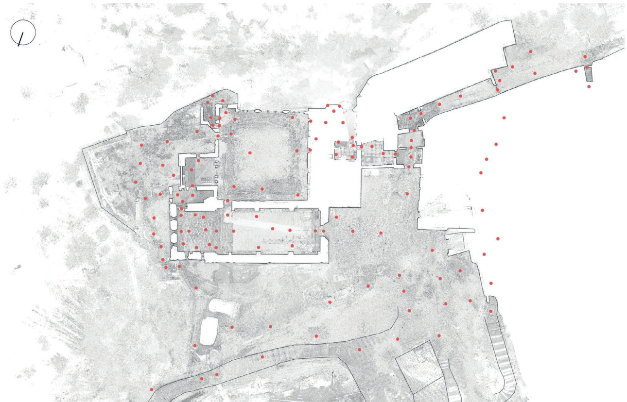
Figure 4 | Planimetric view extract from the point cloud: in red are shown the positions of the single scans made to obtain complete documentation of the monastic complex.
