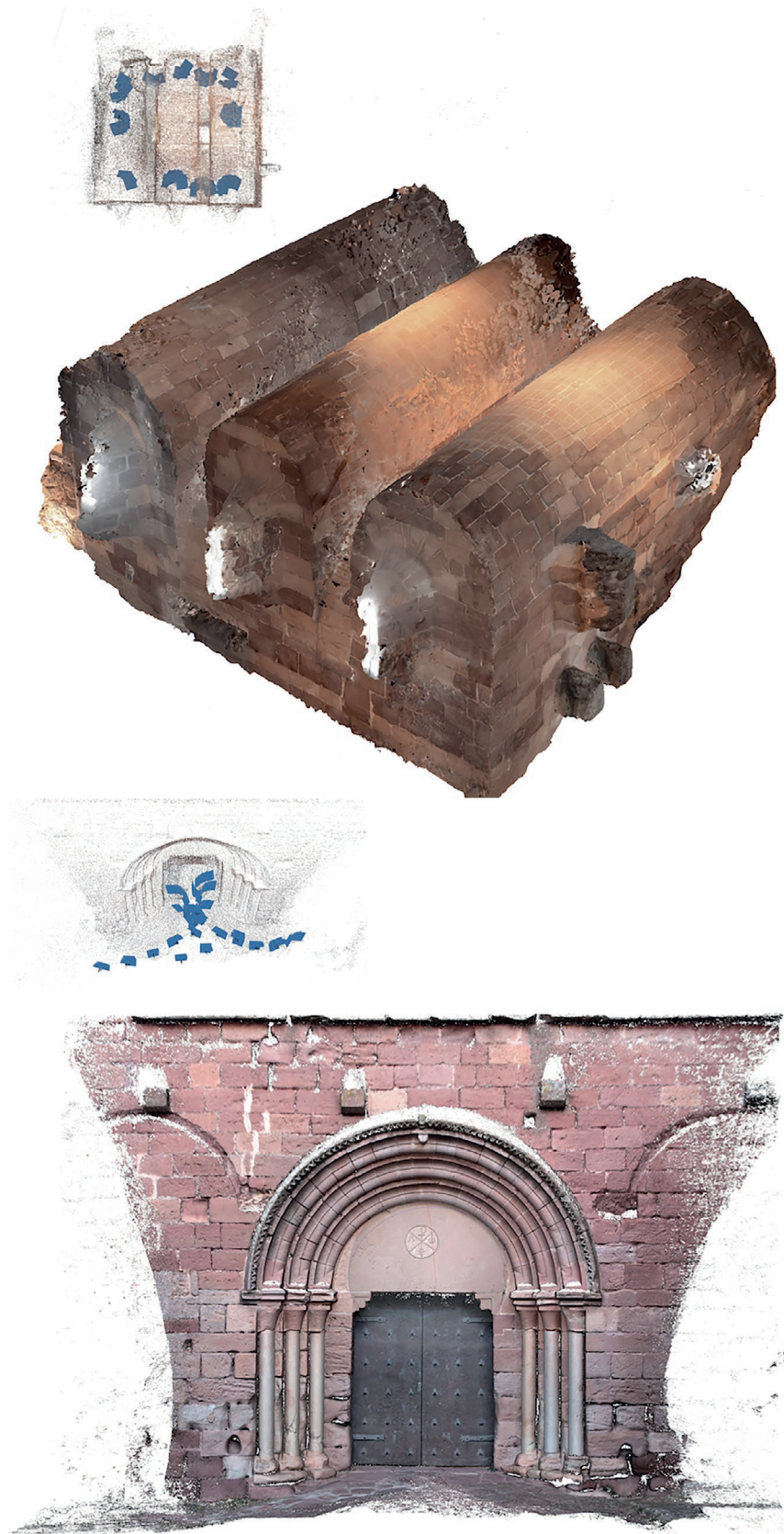
Figure 5 | A photogrammetric model of the crypt (above) and of the church's portal (down). The acquisition schemes underline the different acquisition modes according to the object to be documented.
