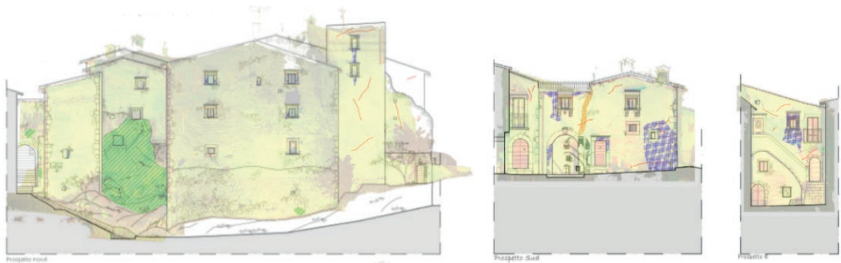
Figure 4 | CAD restitution overlaid with photo-plans for the analysis of decay and instabilities.
