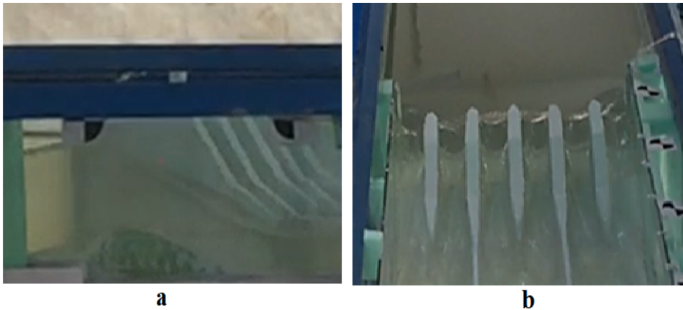
Fig. 2. Approach and entrance of the spillway structure shown during the experiment a) Side view b) Top view
