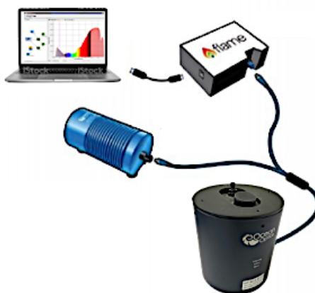
Figure 41 Schematic representation of the set-up using the portable spectrometer fitted with an integration sphere.
