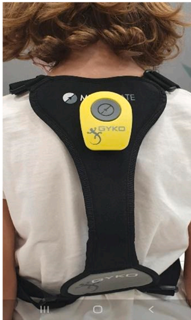
Fig. 1. Placement of the Gyko inertial sensor system on a participant.
