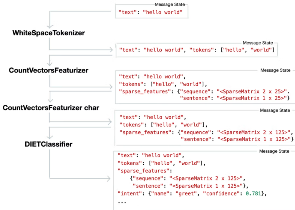
Figure 2.9: Message State in each component of the NLU pipeline
