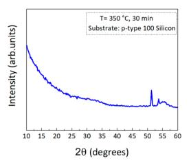
**Figure 10.** Grazing incidence XRD diffractogram of the spin-coated  $ZrO_X$  thin films annealed at 350 °C in air for 30 min and deposited on a silicon substrate.
