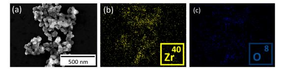
**Figure 4.** (a) SEM image of the  $ZrO_2$  nanoparticles synthesized by microwave irradiation with a further calcination step at 800 °C for 15 min, together with the corresponding EDS maps of Zr (b) and O (c).
