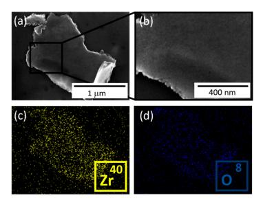
**Figure 8.** (a,b) SEM images of the  $ZrO_2$  particle produced by the combustion synthesis method and after annealing in air at 350 °C for 1 h, together with the corresponding EDS maps of Zr (c) and O (d).
