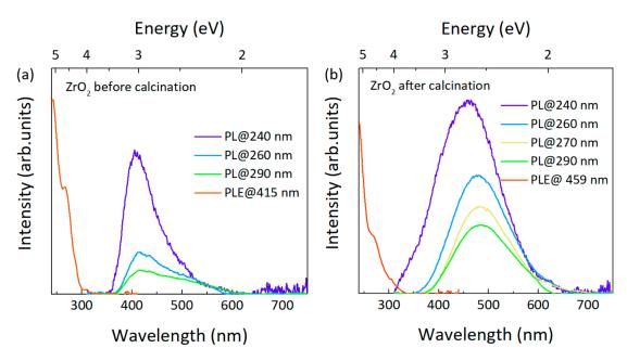
**Figure 6.** PLE/PL spectra acquired at RT on the ZrO<sub>2</sub> nanopowders (**a**) before and (**b**) after a calcination treatment at 800 °C for 15 min.
