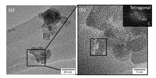
**Figure 9.** TEM images of the  $ZrO_2$  powder produced with solution combustion synthesis and annealed in air at 350 °C for 1 h. (a) Bright-field TEM image of the  $ZrO_2$  nanoparticles and (b) high-resolution TEM images of the  $ZrO_2$  nanocrystals. The inset in (b) shows the FFT images of the area (black square) indicated as C.
