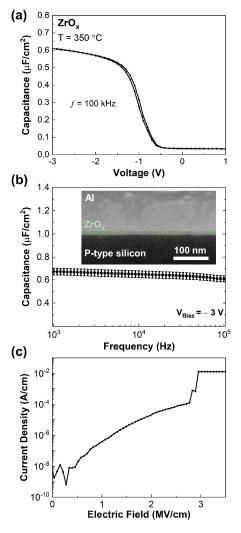
**Figure 11.** Electrical characteristics of solution-based  $ZrO_x$  MIS capacitors produced at 350 °C: (a) typical capacitance-voltage characteristics at 100 kHz; (b) average of capacitance versus frequency characteristics, and the inset shows the cross-section SEM of the devices; (c) typical leakage current density versus the breakdown field.
