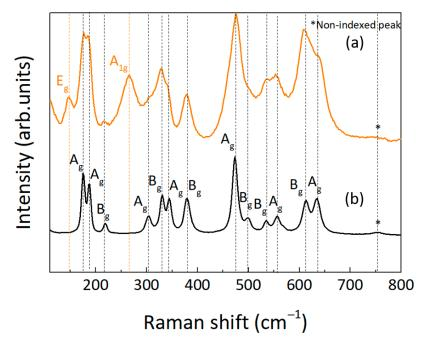
**Figure 2.** Raman spectra of the synthesized ZrO<sub>2</sub> nanopowders: (a) before and (b) after calcination at 800 °C for 15 min. The black and orange vertical dash lines represent the expected frequencies for the monoclinic and tetragonal ZrO<sub>2</sub>, respectively, and according to [77,79,81].
