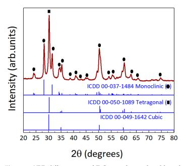
**Figure 7.** XRD diffractogram of  $ZrO_2$  powder produced by solution combustion synthesis and annealed in air at 350 °C for 1 h (represented in red). For comparison, the simulated monoclinic, tetragonal and cubic zirconia structures are also presented.
