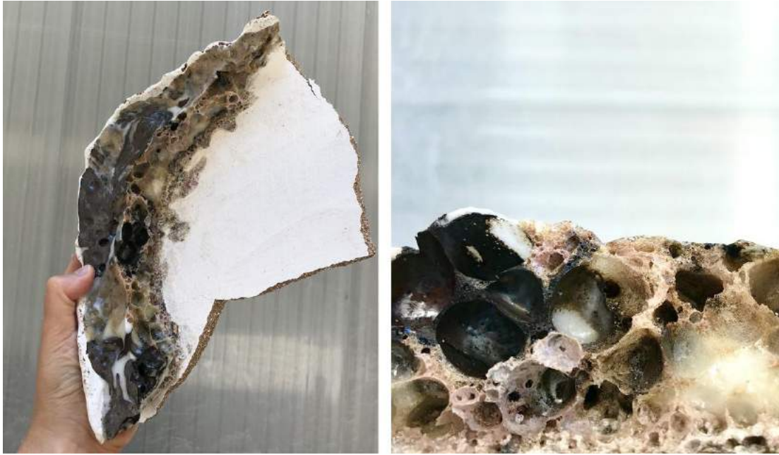
Figure 42 – Fragments of mixed glazes in cross cat.
