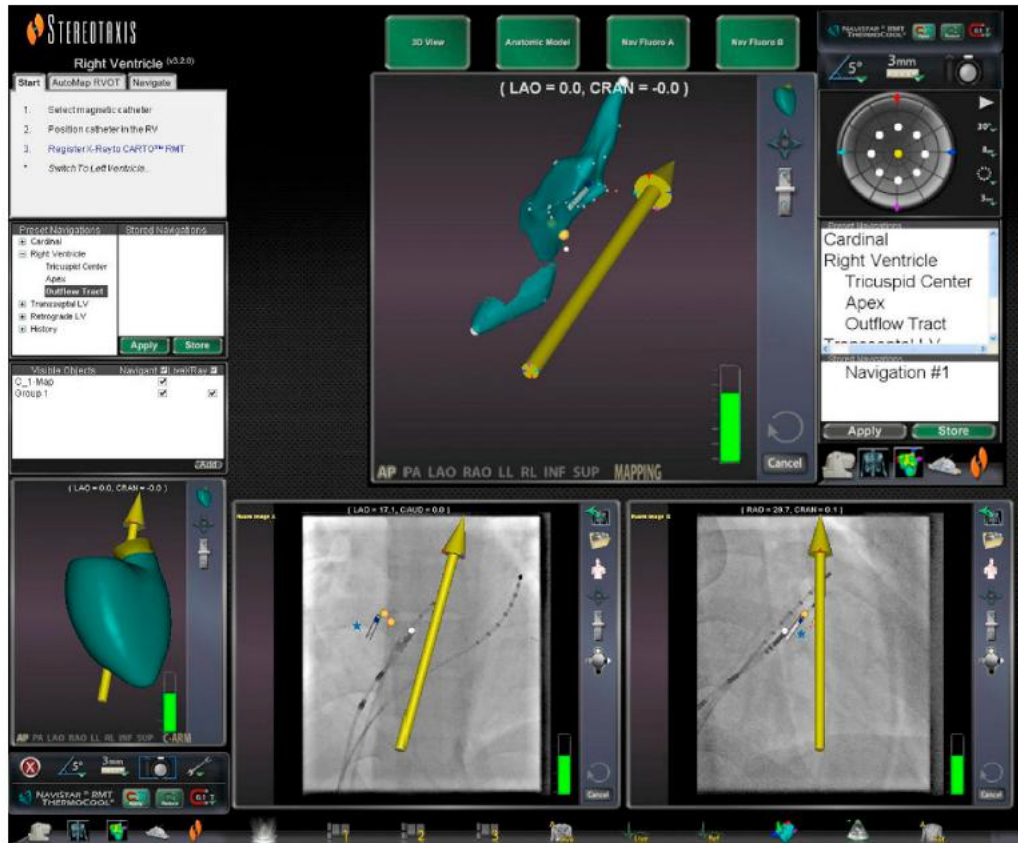
Figure 1 Reference fluoroscopic images on the Navigant workstation in right and left anterior oblique views showing the position of the ablation catheter (blue star) in real time without need for further fluoroscopy; MNS automatic vector indicating the right ventricular outflow tract (yellow vector) and the His bundle (yellow dots).
