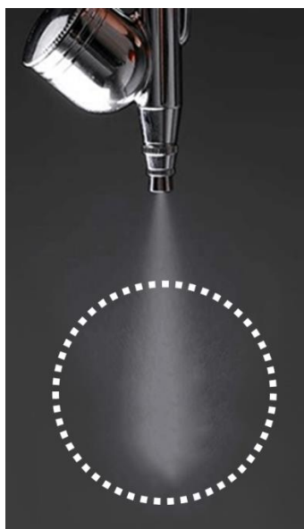
Figure 1.14. Representation of the spray-casting technique. Highlighted the aerosol part of the sprayed solution.
