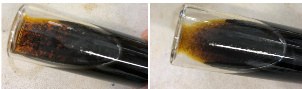
Figure C.3.2. Dispersion of polymer 11 with 7.5% of MWCNTs in a solution of \text{CHCl}_3 :toluene with a 5:1 ratio. Left: Blend just after preparation; Right: Blend after 6 hours of sonication at 40^\circ\text{C} .
