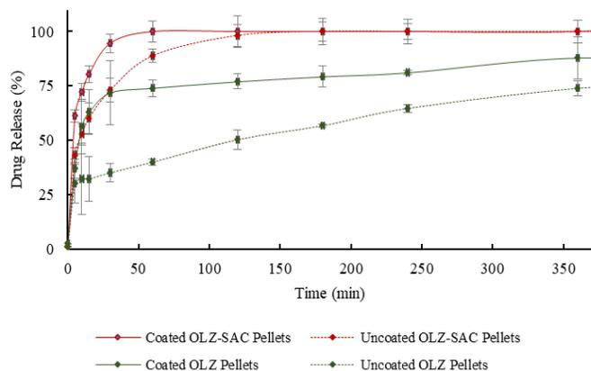
**Figure 1: Dissolution profiles of coated and uncoated pellets with OLZ and with OLZ-SAC**
