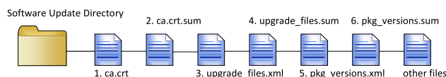
FIGURE 10. Software update directory – Contains the files that are to be pushed to the gateway in case of an update. 1&2: The security certificate of the gateway and its cryptographic hash. 3,4,5&6: Store the version numbers of files in the directory and their associated cryptographic hash. Certificates files can be replaced in this folder and hashes recomputed by adversaries.
