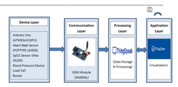
Figure 1. Architecture of Smart Maternal Monitoring Device..
