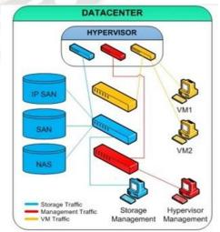
Figure 1 Components in Virtual Data Center
