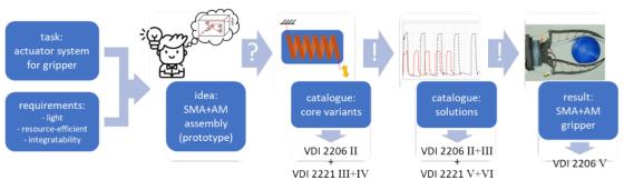
Figure 6. Example of the simplified development of an SMA+AM gripper using the guideline integrated into the VDI framework
