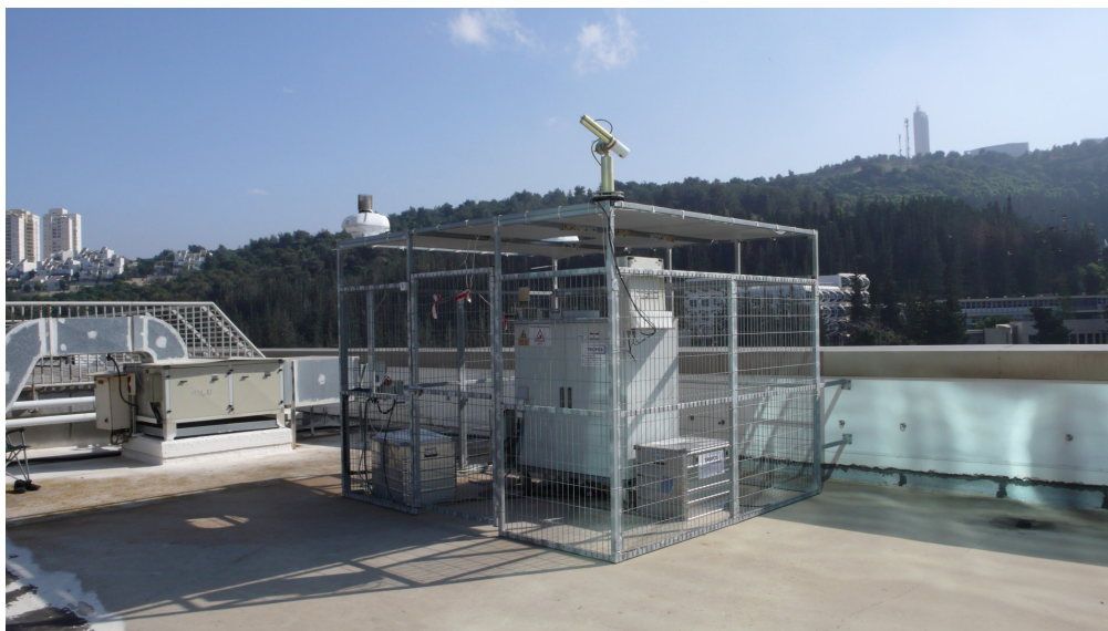
Figure 1. Polly XT on the rooftop platform at Technion, Haifa, in March 2017. The instrument is placed inside a protective cage to avoid unauthorized access. On top of the cage, an air-safety radar is monitoring the sky for airplanes, and an AERONET sun photometer is measuring the aerosol optical thickness. In the background, the northern tips of the Carmel mountain range and the tower of the University of Haifa can be seen.
