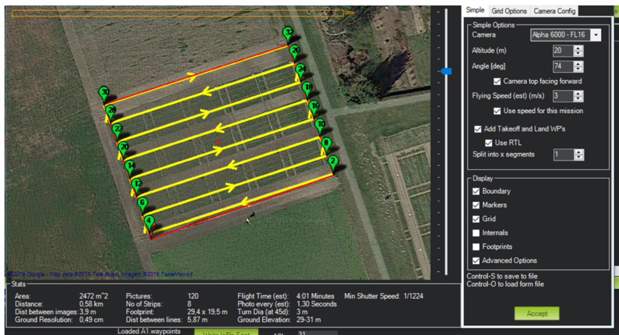
Figure 5. The actual flight route of UAV for the nadir imagery.
