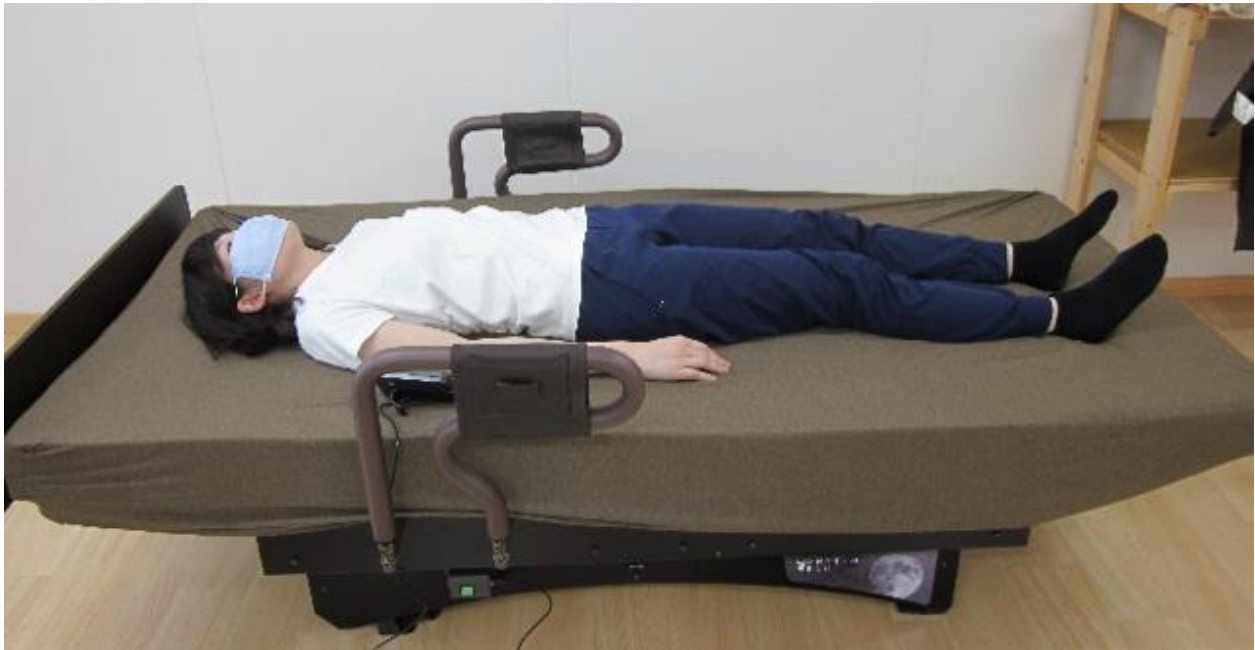
Figure 1. An electric sway bed (dimensions: 1900 × 900 × 500 mm (length × width × height)), powered by an electric motor, with seven sway speed settings. The motorized device was set to sway the student vertically by \pm 2 cm for a total of 4 cm. In this study, the level 2 (0.64 Hz) sway speed was used.
