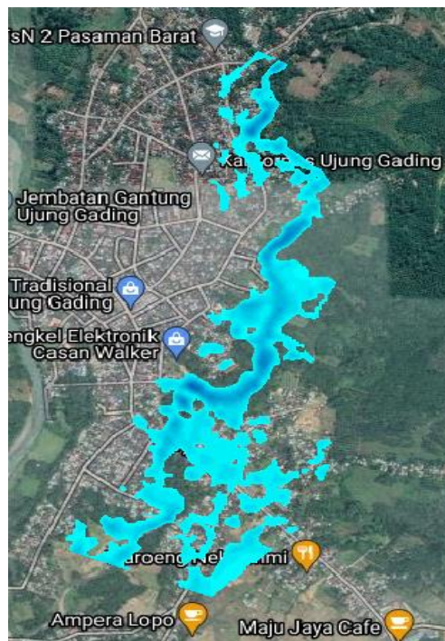
Figure 10. River Overflow Area 5 year Return Period.
