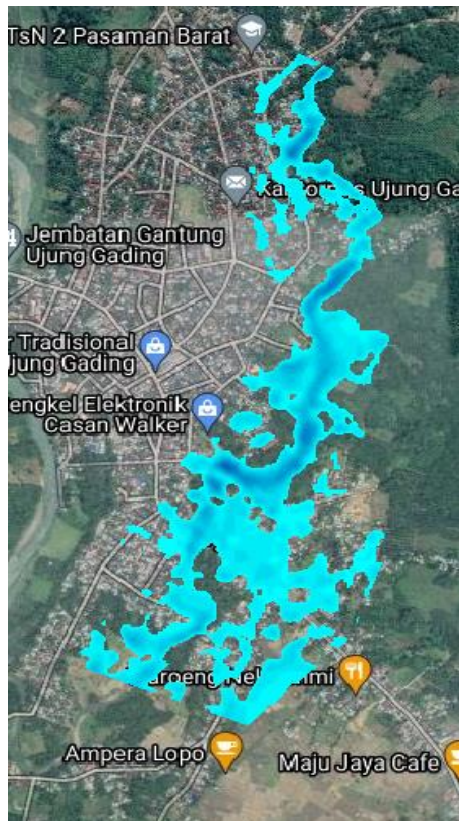
Figure 11. River Overflow Area 10 year Return Period.
