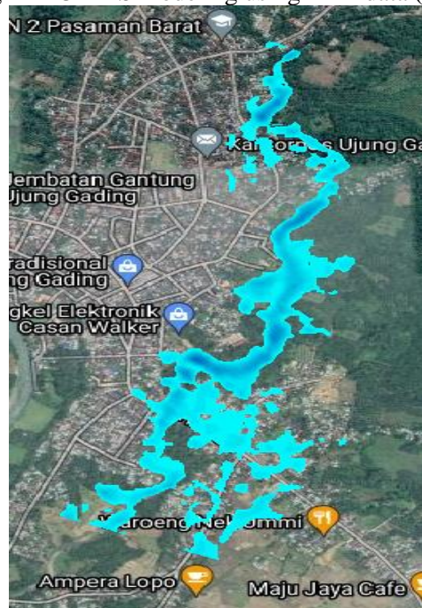
Figure 9. River Overflow Area 2 year Return Period.
