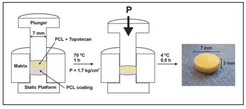
Figure 5. Melt molding compression technique
