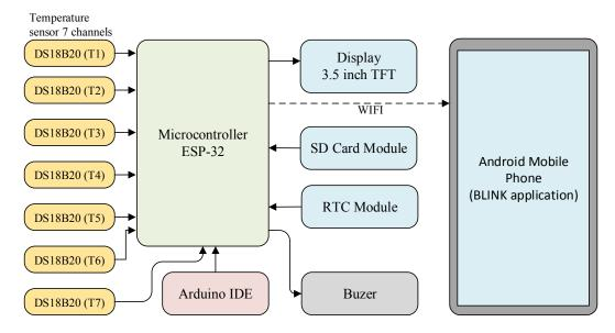
FIGURE 1. block diagram of the entire system of the blood bank temperature distribution monitoring device.
