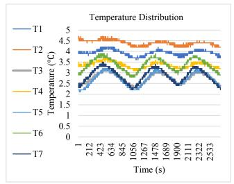
**Figure 2.** Line graph of temperature distribution T1-T7 on a temperature monitoring device at blood bank temperature setting (4°C).
