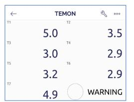
Figure 7. Blynk application display for wireless temperature monitoring
