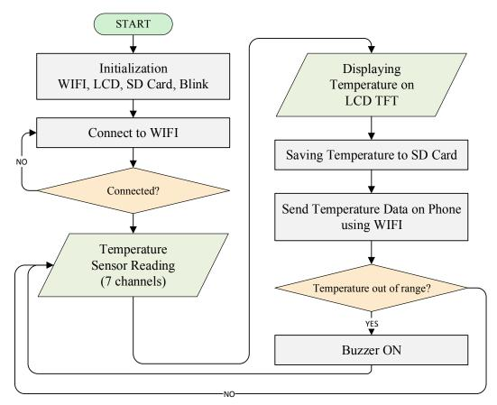
FIGURE 2. Flowchart of the entire temperature parameter measurement.
