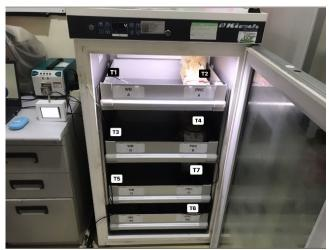
**FIGURE 3.** Location of measurement points T1, T2, T3, T4, T5, T6 dan T7 using the Blood bank.
