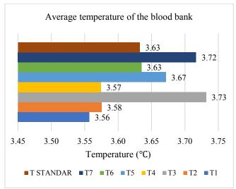
**Figure 1.** Comparison of measurements of T1, T2, T3, T4, T5, T6 and T7 between temperature monitoring devices and standards on blood bank temperature setting  $(4^{\circ}C)$ .
