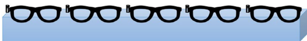
FIGURE 1 Schematic drawing of the Clouclips mounted on spectacle frames attached to a solid, portable board for inter-device reliability measures. Diagram not to scale
