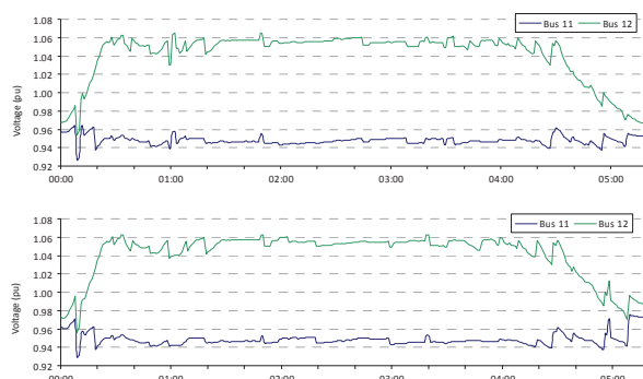
Figure 4: Voltage Profiles for single step OPF formulation (Top) and Extended Control Horizon (bottom).
