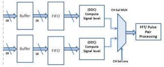
Figure 5. Data flow architecture for overlapping.
