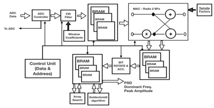
Figure 3. Proposed architecture for on-board frequency domain analysis.
