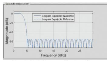
Figure 4. Magnitude response of equiripple filter.
