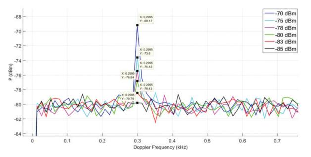
Figure 8. Field test signal with 1024 point FFT and 25 % overlapping.
