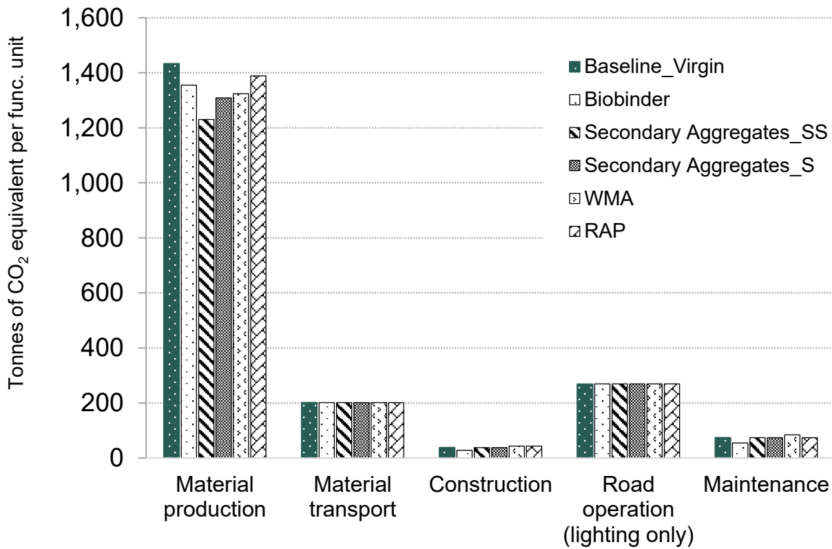
Figure 6: Sensitivity of the embodied carbon of a functional unit of study (baseline highlighted in 'green') to the integration of low-carbon alternative materials and technology
