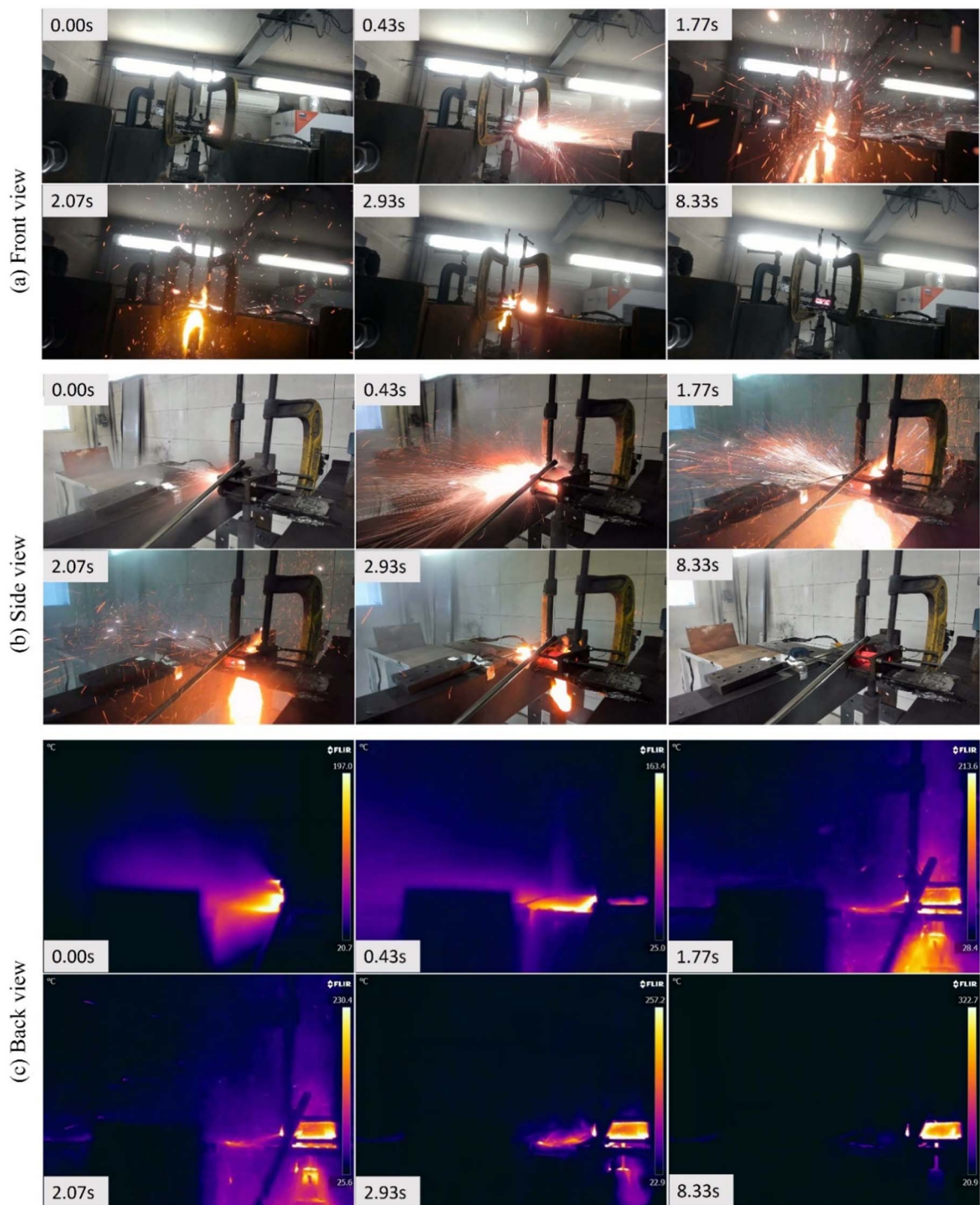
Figure 5. Evolution of fire behaviour of test 1 at 100% SOC. (a) Front view, (b) side view, and (c) back view from the IR camera.
