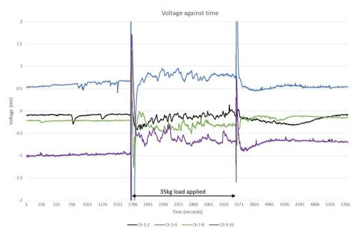
**Figure 4.** Electrical activity (recorded on Ch 1–2, Ch 3–4, Ch 7–8, Ch 9–10) before, during and after load (35 kg) was evenly distributed across insole.
